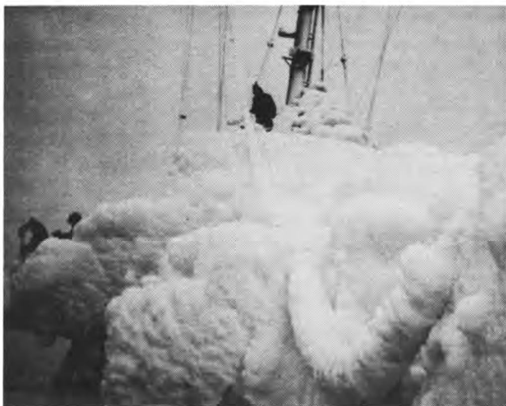
The good old days? Crewmen battle tons of ice sheathing caused by freezing spray on the USCGC OWASCO during patrol on Ocean Station "Bravo" in the stormy Labrador Sea. This severe icing condition was threatening to get out of hand and endanger the ship's stability. U.S. Coast Guard Photo.
